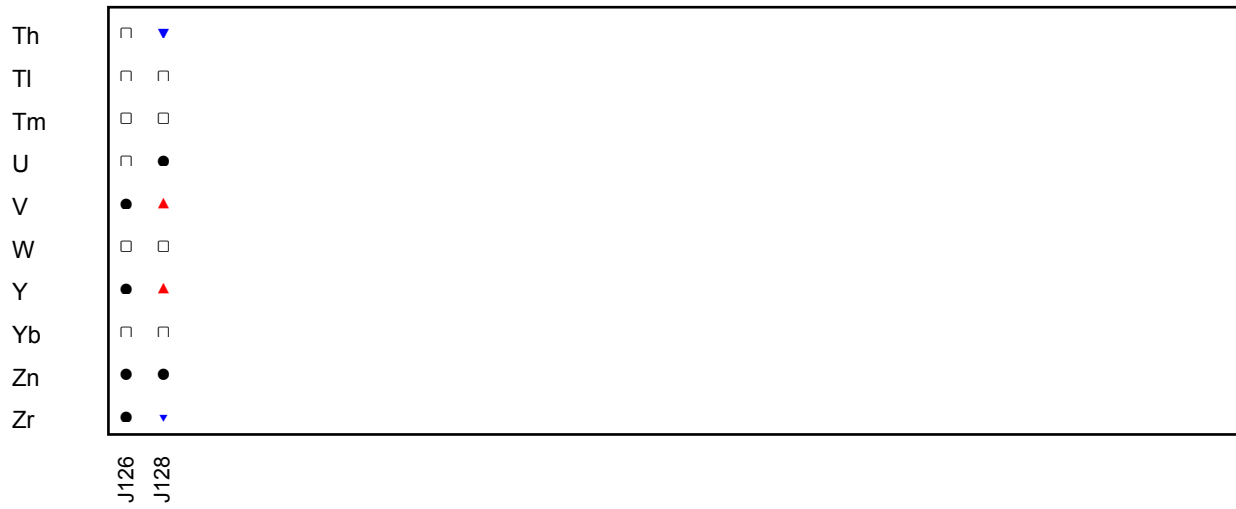
Figure 3: GeoPT47A - Silty soil, NES-1. Multiple z-score charts for laboratories participating in the GeoPT47 A round. Symbols indicate whether or not an elemental result complies with the -2 < z < +2 criteria (see key).
