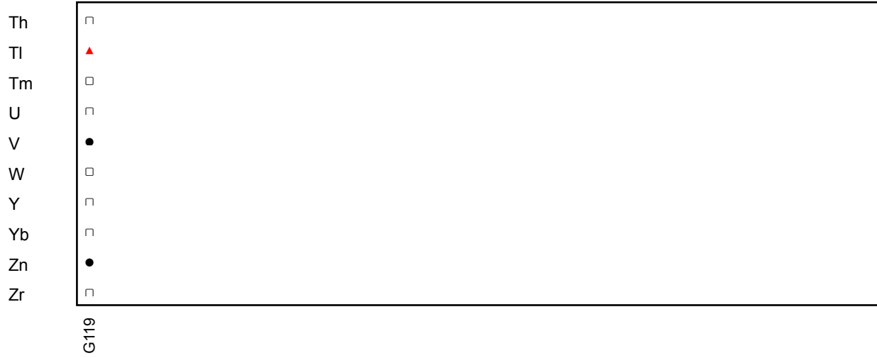
Figure 3: GeoPT46A - Phosphate rock, POLC-1. Multiple z-score charts for laboratories participating in the GeoPT46 A round. Symbols indicate whether or not an elemental result complies with the -2 < z < +2 criteria (see key).
