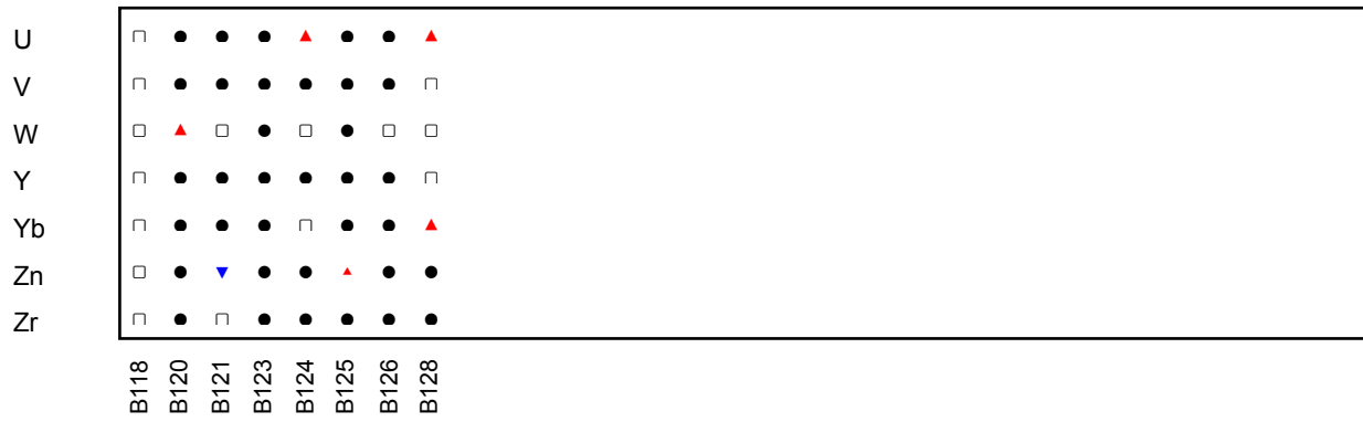
Figure 3: GeoPT43 - Dolerite, ADS-1. Multiple z-score charts for laboratories participating in the GeoPT43 round. Symbols indicate whether or not an elemental result complies with the -2 < z < +2 criteria (see key).
